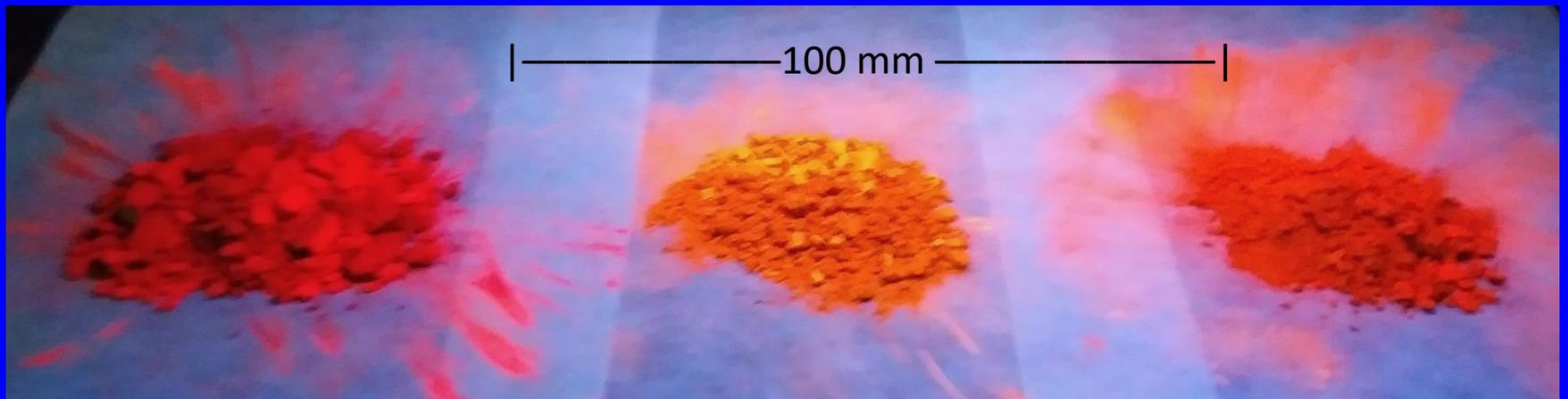
Photoluminescence from RaPSi can be tuned across the whole of the visible spectrum by control of the etching parameters
