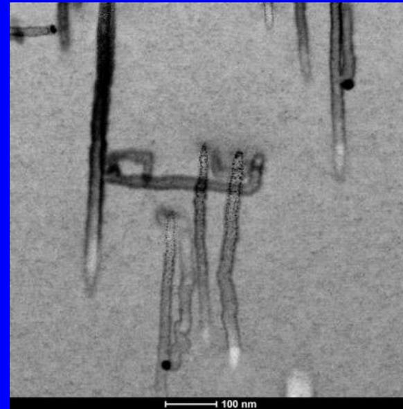
Using electroless etching in the ReEtch process it is now feasible to generate porous silicon powders in quantities limited only by the size of your beakers from metallurgical grade Si. Furthermore problems with thermal budget and foaming can be alleviated by this new  $V_2O_5 + H_2O_2 + HF$  method. Foaming is reduced and homogeneity is enhanced by addition of acetic acid.
