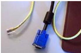
These two cables should be on the table waiting for you. The large cable connects the computer to the projector and the small USB cable connects the computer to the Smart Podium.
