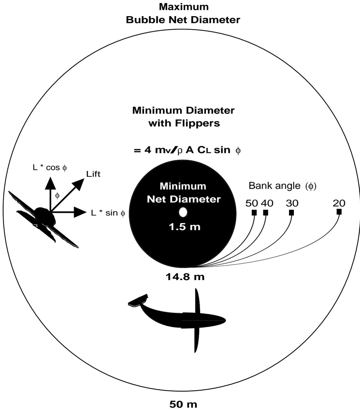
Fig. 6. Calculated and observed turning performance of the humpback whale (*Megaptera novaeangliae*). The calculated minimum turning diameter (14.8 m) for a 9 m whale is shown by the outer margin of the black circle, based on the equation shown. The margins of the turn for various bank angle are shown by curved lines. The minimum and maximum diameters of bubble nets are shown by the margin of the central white circle and the outer white circle, respectively. The lift (L)
