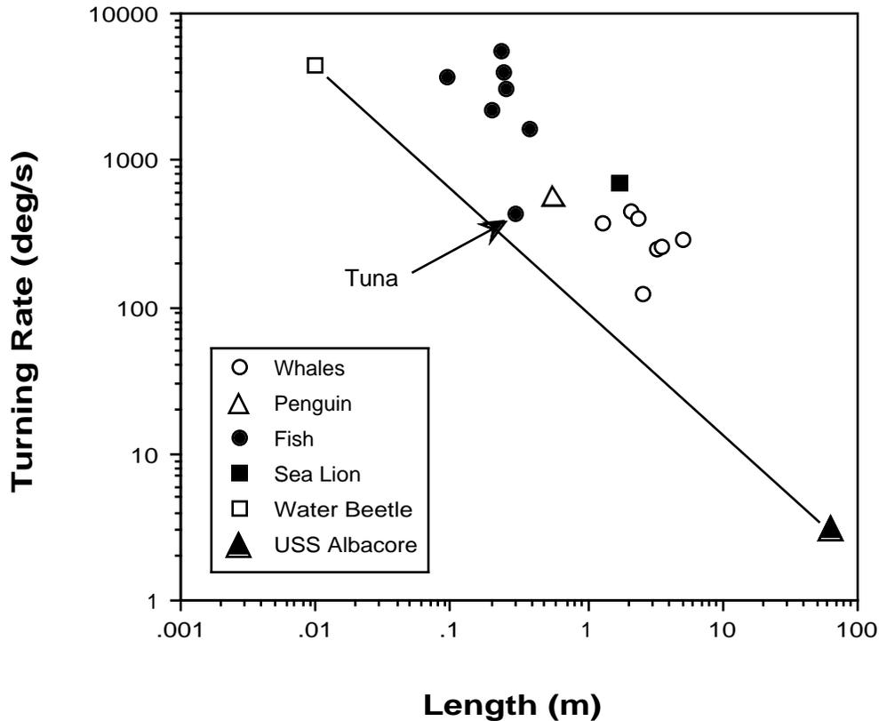
Fig. 7. Comparison of turning rate with respect to size. The line connects the beetle and submarine which both have inflexible bodies. The value for relatively stiff tuna approaches the line. Data from Webb, 1976, 1983; Hui, 1985; Miller, 1991; Blake et al., 1995; Fish, 1997.
