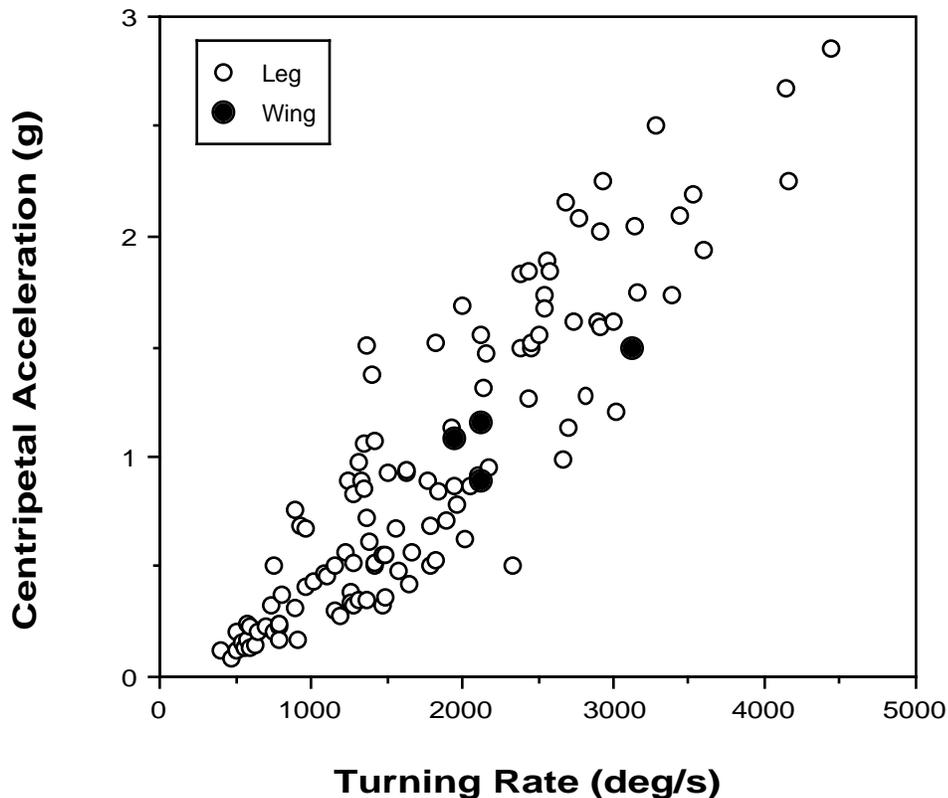
Fig. 5. Relationship between centripetal acceleration and turning rate for whirligig beetles. Open circles represent swimming by rowing of the legs; closed circles represent turns executed by drag from the elytra and vectored thrust produced by a sculling wing.
