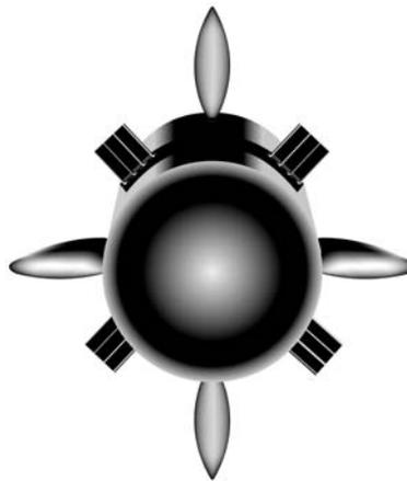
Fig. 4. Front view of biomimetic robot showing position of the control surfaces. The high-aspect ratio fins are located at positions  $0^\circ$ ,  $90^\circ$ ,  $180^\circ$  and  $270^\circ$  and small-aspect ratio fins are located at positions  $45^\circ$ ,  $135^\circ$ ,  $225^\circ$ , and  $315^\circ$ .
