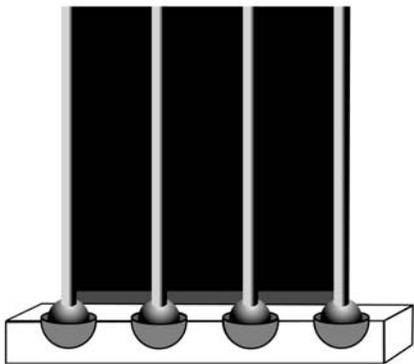
Fig. 3. Close-up of low-aspect ratio pectoral fin for biomimetic robot. The fin is composed of a flexible membrane supported by four rigid rods. The base of each rod has a spherical end to form a ball-and-socket joint for multi-axial movement. Artificial muscles inserting at the base of the rods will control the movements in a coordinated manner.
