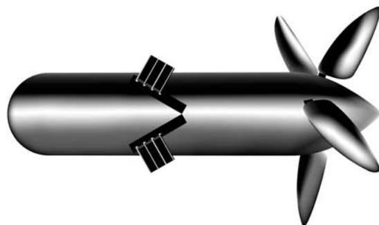
Fig. 2. Biomimetic robot with high-aspect ratio and low-aspect ratio fins for propulsion and maneuvering. The high-aspect ratio fins located posteriorly are based on the flipper designs of penguins and marine mammals. The low-aspect ratio fins are located around the center of gravity. These fins are based on the pectoral fins of fishes. The low-aspect ratio fins are oriented at an angle. These fins may be folded into slots to reduce drag.
