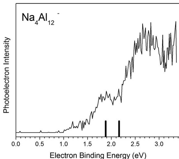
FIG. 15. Photoelectron spectrum of the  $\text{Na}_4\text{Al}_{12}^-$  cluster anion. The overlaid stick spectra indicate the calculated transitions from the ground state of the  $\text{Na}_4\text{Al}_{12}^-$  cluster anion to the ground and first excited states of the  $\text{Na}_4\text{Al}_{12}$  neutral cluster.
