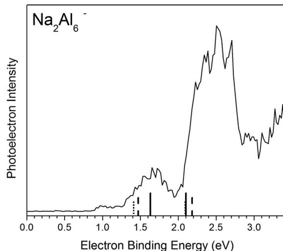
FIG. 3. Photoelectron spectrum of the Na<sub>2</sub>Al<sub>6</sub><sup>-</sup> cluster anion. The overlaid stick spectra indicate the calculated first two transitions from the Na<sub>2</sub>Al<sub>6</sub><sup>-</sup> anion to its corresponding neutral cluster. (Solid sticks: isomer 1; dashed sticks: isomer 2; dotted sticks: isomer 3.)
