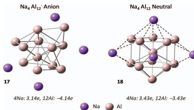
FIG. 14. The lowest energy isomers of the  $\text{Na}_4\text{Al}_{12}^-$  cluster anion (**17**) and the  $\text{Na}_4\text{Al}_{12}$  neutral cluster (**18**). The gray spheres represent aluminum atoms and the purple spheres represent sodium atoms. The calculated Natural Population Analysis (NPA) charges are given in italics below each isomer.
