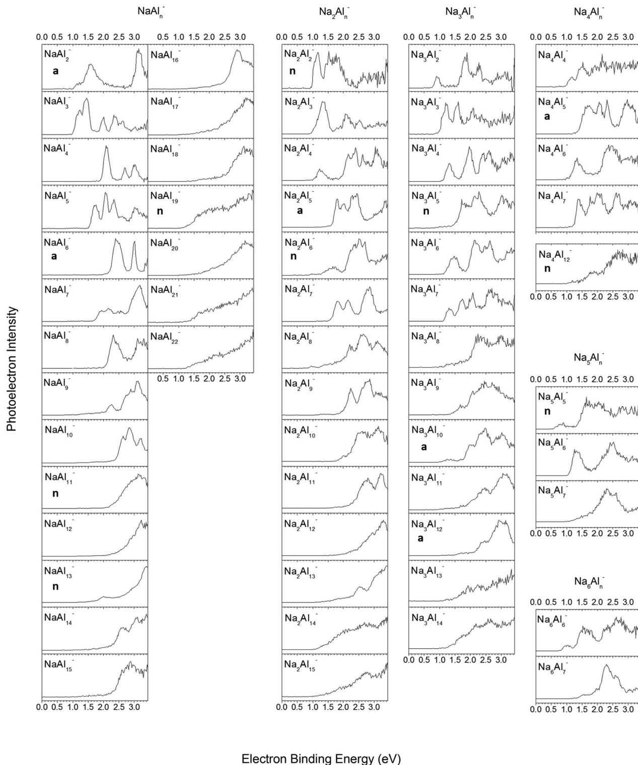
FIG. 1. Photoelectron spectra of  $\text{Na}_m\text{Al}_n^-$  cluster anions, ( $m = 1, n = 2\text{--}22$ ;  $m = 2, n = 2\text{--}15$ ;  $m = 3, n = 2\text{--}14$ ;  $m = 4, n = 4\text{--}7$  and  $12$ ;  $m = 5, n = 5\text{--}7$ ;  $m = 6, n = 6\text{--}7$ ). Species with closed shell neutrals are marked by “n,” and those with closed shell anions are marked by “a.” Note that the valence electrons for these closed shell clusters, based on the jellium model, are 8, 18, 20, 34, 40, and 58.
