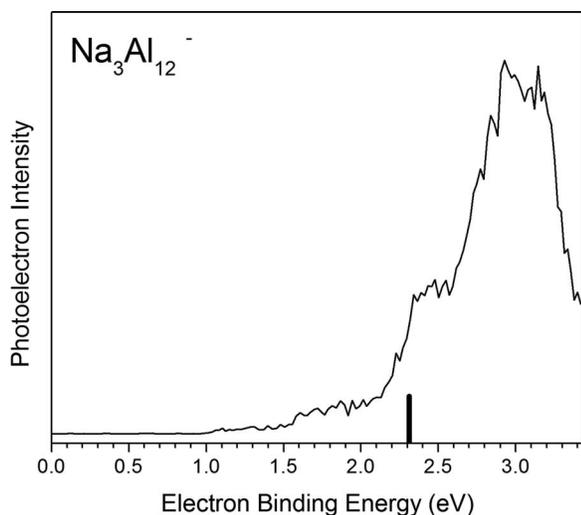
FIG. 12. Photoelectron spectrum of the  $\text{Na}_3\text{Al}_{12}^-$  cluster anion. The overlaid stick spectra indicate the calculated transitions from the ground state of the  $\text{Na}_3\text{Al}_{12}^-$  cluster anion to the ground state of the  $\text{Na}_3\text{Al}_{12}$  neutral cluster.
