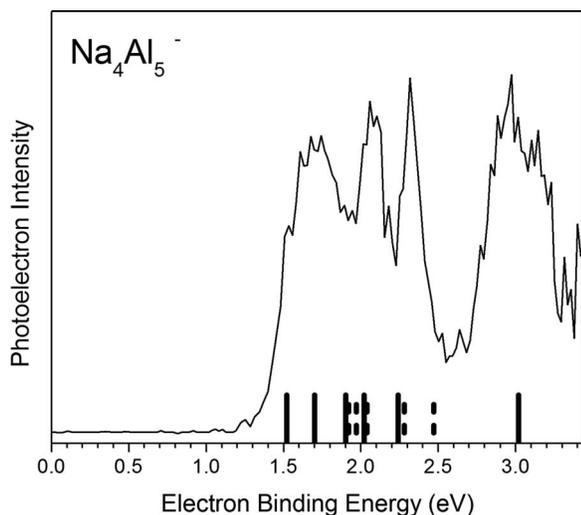
FIG. 6. Photoelectron spectrum of the  $\text{Na}_4\text{Al}_5^-$  cluster anion. The overlaid stick spectra indicate the calculated low energy transitions from the  $\text{Na}_4\text{Al}_5^-$  anion to its corresponding neutral cluster. (Solid sticks: isomer 7; dashed sticks: isomer 8.)
